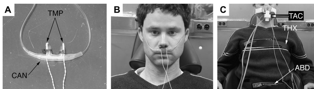
Figure 1 Subject setup. Panel A shows the cannula (CAN) that is attached to the piezoelectric pressure sensor (not shown) and the 2 thermistors (TMP). Small zip-ties are used to fasten the thermistors to each orifice of the cannula. Panel B shows the CAN and TMP apparatus attached to a subject. The remaining measurement devices are shown in panel C . The thoracic belt (THX) is secured below the arms, whereas the abdomen belt (ABD) is secure around the midsection at the level of the naval. The pneumotachometer flow head (TAC) is attached to the mask via a short flexible tube.
